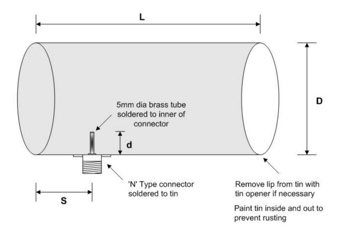
Comparative tests indicate that antenna provides approximately 11dB gain over a dipole
